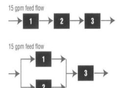
reduce build up of concentrated materials at the membrane surface. When several membranes are being used, the arrangement of these membranes is crucial in maintaining proper flow velocities. This arrangement must be checked against other related factors such as higher pumping costs, recycle flow, etc.
