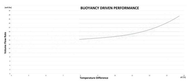
The above is based on the house size test facility monitored by Imperial College London. Buoyancy driven ventilation through single unit delivered 28m3/h of fresh air at temperature difference (the driving factor) of 13 degree C.
