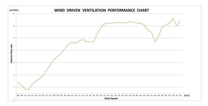
The above wind tunnel tests demonstrate the performance of the cowl at wind speeds between 0.8 and 7m/s (2.9 to 25 km/h). At wind speed 2.7m/s the ventilation rate raises to 5m<sup>3</sup>/h, increasing gradually to 11m<sup>3</sup>/h at the wind speed of 3.2m/s (the average wind speed in built up areas). The cowl is designed to throttle the flow at higher wind speeds to avoid discomfort.
