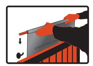
7. Position Radklips on hooks. If needed, roll more or trim bottom.
