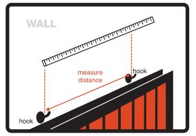
Flatten creases with thumb - does not need to be perfectly flat. Attach the hooks to the wall behind the radiator close to the top.
