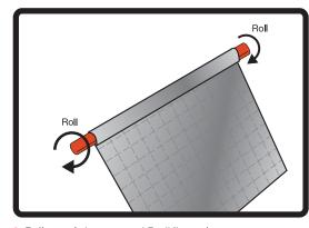
6. Roll top of sheet around Radklips at least once to secure.
