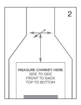
A Standard Size Chimney Umbrella has been designed to fit all square and rectangle flue sizes between 200mm x 200mm and 380mm x 380mm.
