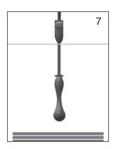
CHIMELLA'S display handle has been designed so it can always be on view at a position of your choice. Simply hold the release button in one hand and pull down gently on the display handle with the other hand and extend down.
