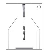
Push the extended display handle up towards the release button and pull the CHIMELLA down and out of the fireplace opening. As any dirt is now safely and cleanly held in the canopy you can take it away and dispose of it into a bin efficiently with NO MESS.
