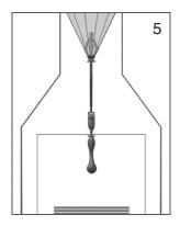
When the extendable shaft reaches its full extension the patent pending technology allows the chimney blocker canopy to open fully and hold itself in place.
