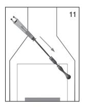
Hold the nest area at the bottom of the canopy in one hand and the button handle in the other. Push the nest area towards
