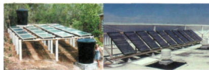
Left: A basin-type solar distiller array with two storage tanks in Kona, Hawaii. Right: A tilted solar still with panels measuring 36-x78-inches; each are connected in tandem to increase product water yield at a Tucson, Ariz., community college.
