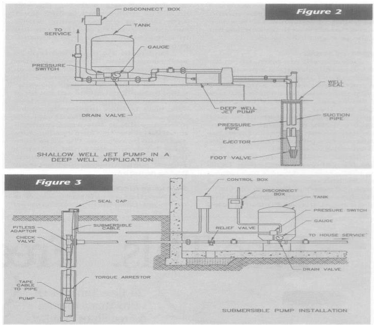
Because of its multiple stages, the submersible pump generally delivers higher pressure than jet pumps of the same horsepower. This type of pump is normally selected for deeper wells; and, with their high capacity, increased pressure and quiet operation, they make an ideal selection for home and commercial use.
