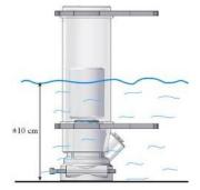
There will be a spluttering from the tap as air is purged from the system. Once water is running freely this tap can be closed.
