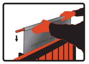
Position Radklips on wall brackets. If needed, roll more or trim bottom.
