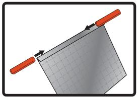
4. Slide on at least two Radklips over the fold.
