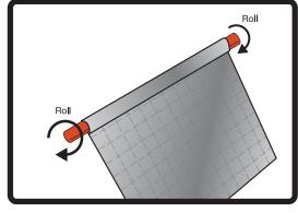
6. Roll top of sheet around Radklips at least once to secure.
