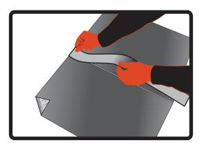
8. If you need to use Radstik joining tape: Place two sheets of Radflek side by side, printed side down. Stick Radstik onto the unprinted side over the join. Do NOT use Radstik to stick Radflek to the wall or radiator.
