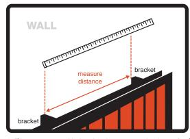
1. Flatten creases with thumb - does not need to be perfectly flat. Measure distance between radiator wall brackets behind radiator.
