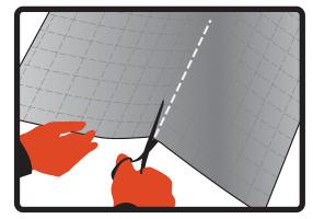
2. Cut Radflek sheet to width between wall brackets.
