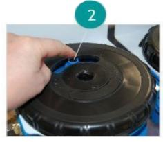
2. Press the pressure release button on all housings (2).
