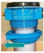
3. Unscrew the bowl locking ring by turning to the left. To release the ring, it may be necessary to give the spanners handle a rap with the heel of your hand
