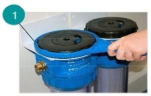
1. Position a suitable receptacle under the system to catch residual water. Then using the plastic spanner (1) supplied with the system to shut off the water supply by rotating the ring of the housing until the arrows on all of the housings point to 'OFF' or 'BYPASS'.
